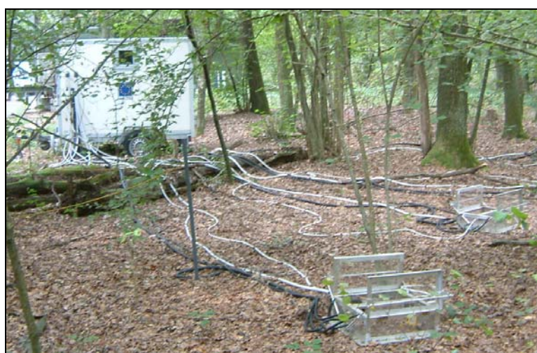
Pic. 1: Chamber system to measure NO & NO 2 fluxes from soil at the JRC Ispra forest site.
