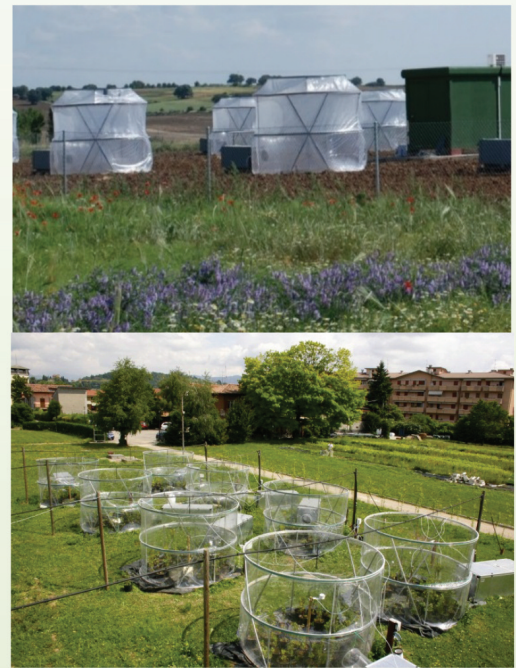
Ozone exposure experiments using open-top chambers in Spain and Italy
