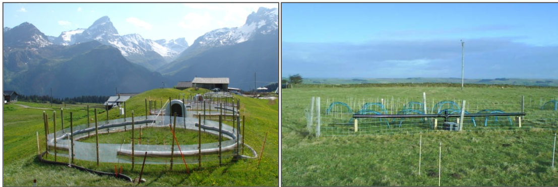
Figure 4.4 Examples of experiments investigating ozone effects on pasture using free air exposure systems (a) At Alp Flix, Switzerland (Photo: S Bassin) and (b) at Keenley, UK (Photo: G Mills).
